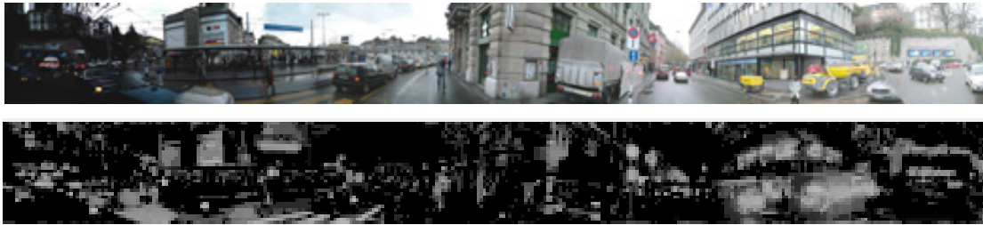
Figure 4 The picture on top shows a typical urban scene and the picture below shows the corresponding saliency map, as generated by Itti and Koch’s saliency-based model of spatial attention. Each salient or conspicuous location in an image or a scene is evaluated with respect to its surrounding.
