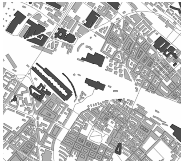
Figure 8: Result of the identification of extraordinary buildings, to handle them separate during map generalisation. Data: VECTOR 25, reproduced by permission of swisstopo (BA057008).
