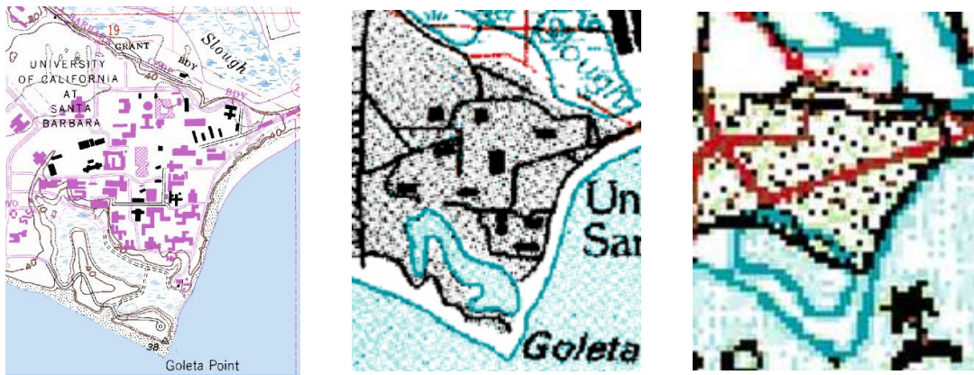
Figure 5. Graphic and Semantic changes of level-of-detail as a function of scale change across standard scales from the topographical map series provided by the U.S. Geological Survey 1 .
