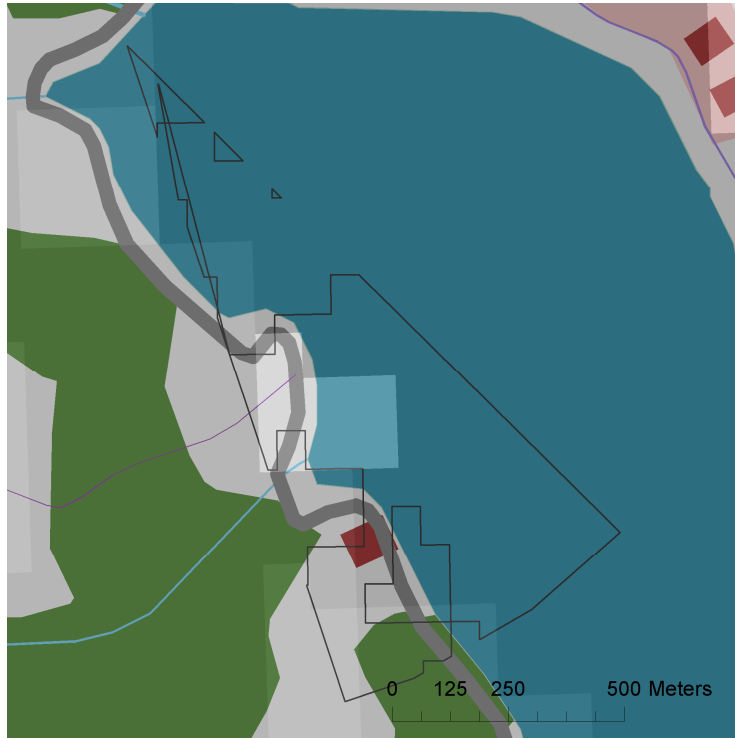
Figure 1. Spatial data for a visible area corresponding to the second image shown in Figure 2 – ©SwissTopo 1:200 000 and Corine data are shown here – note the viewshed is restricted to a range of 1.5km and is calculated using SRTM 90m data
