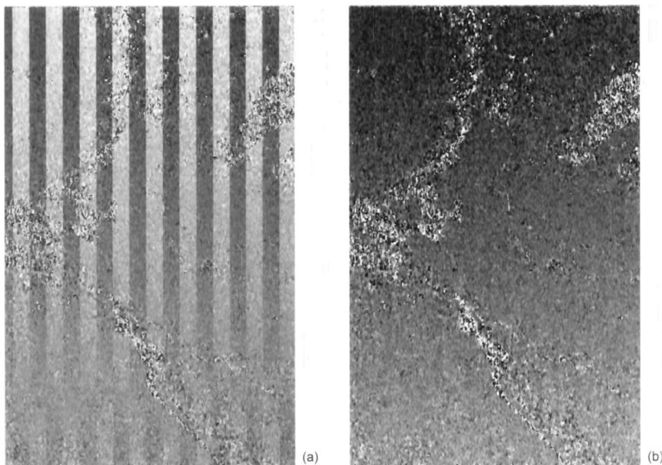
Fig. 12. (a) Difference phase map between the first and third azimuth look. (b) Estimated azimuth misregistration map scaled to  $\pm 1$  azimuth raw data sample.
