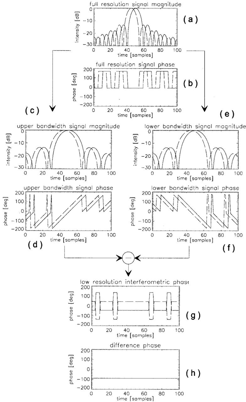
Fig. 4. Simulation of full resolution and bandfiltered signals for coregistration by spectral diversity. The solid line relates to the first interferometric channel and the dashed line to the misregistered second channel.
