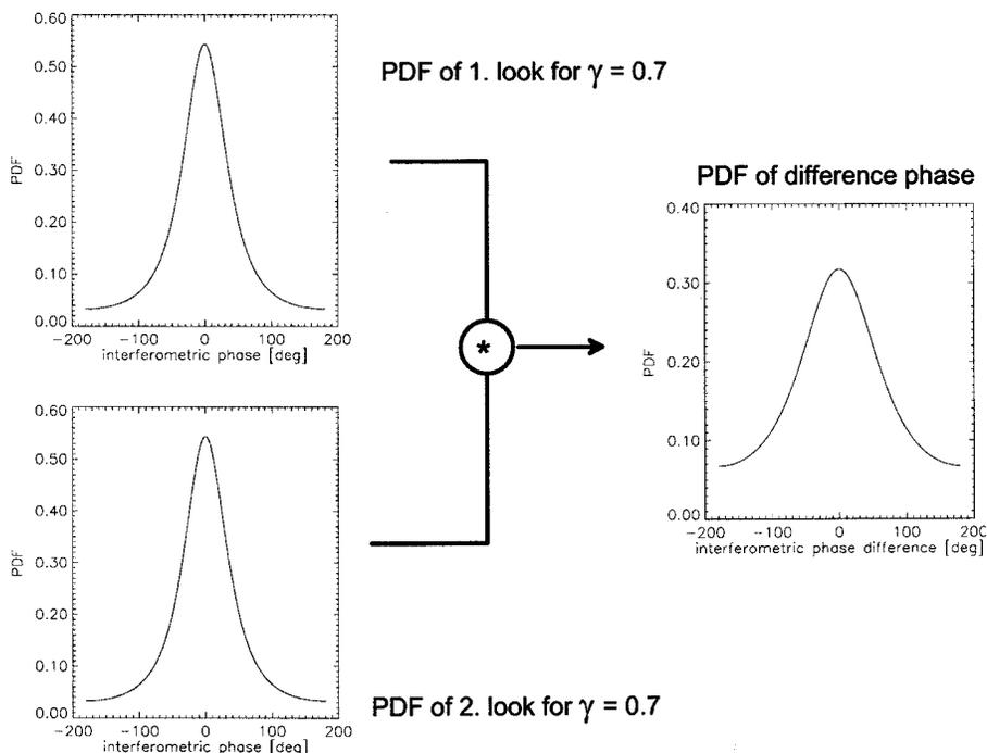
Fig. 5. Probability density function (PDF) of the difference phase as the convolution of the PDFs of the interferometric phase of the two looks.
