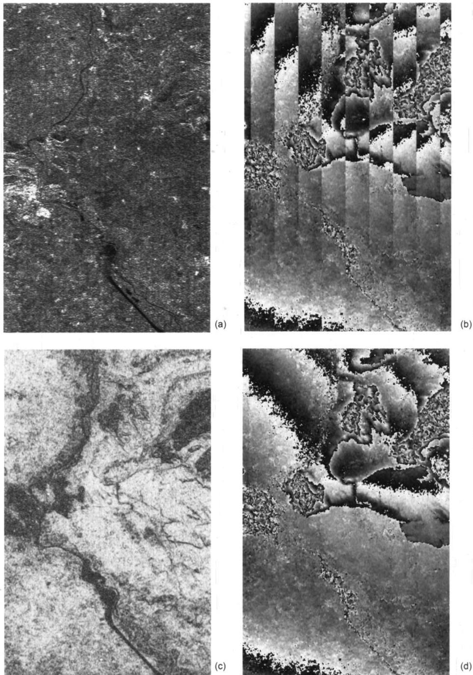
Fig. 11. Simulated ScanSAR data based on an ERS tandem pair (azimuth is horizontal, range vertical). (a) Intensity image processed to four azimuth looks and six range looks. (b) Interferometric phase of one azimuth look with inaccurate burst alignment (eight complete bursts are shown). (c) ScanSAR coherence map. (d) Interferometric phase of one azimuth look after accurate azimuth coregistration.
