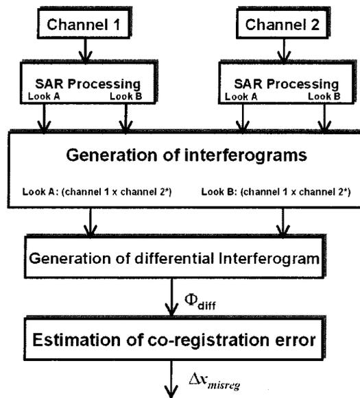
Fig. 3. Block diagram of the proposed spectral diversity approach for interferometric image coregistration.
