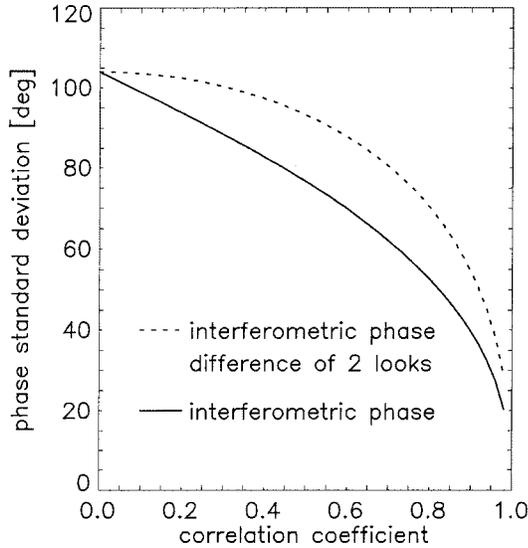
Fig. 6. Standard deviation of the interferometric phase and of the interferometric phase difference as a function of the correlation coefficient.
