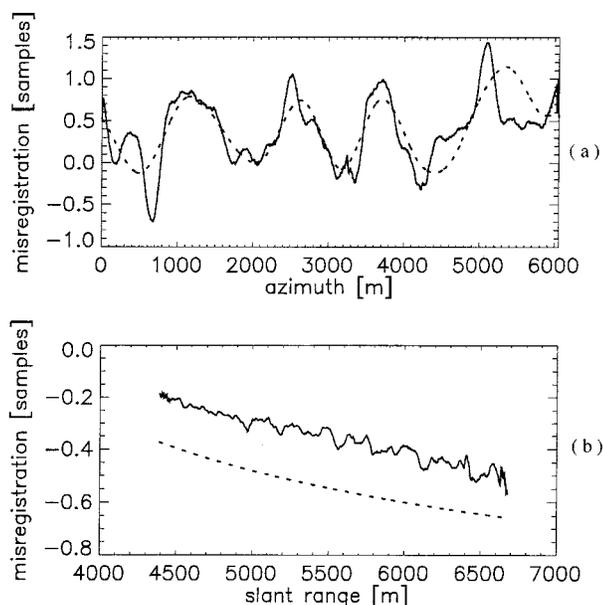
Fig. 9. (a) Estimated azimuth misregistration using the spectral diversity technique and a conventional method (dashed line). (b) Estimated range misregistration and theoretical values (dashed line) according to the measured tracks.
