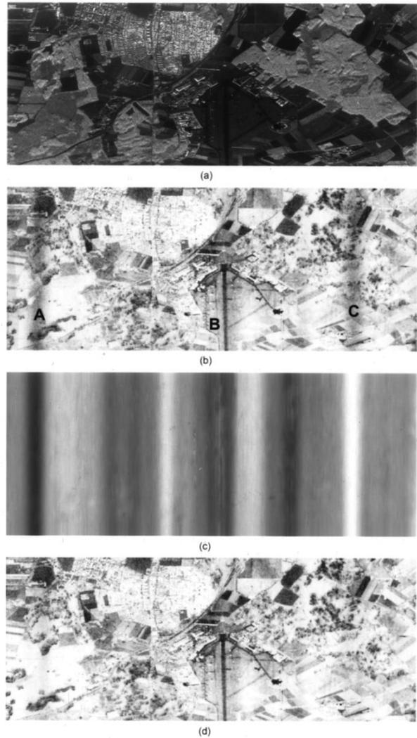
Fig. 8. E-SAR image of Oberpfaffenhofen airfield. (a) L-band, HH-polarization, 4-look intensity image. (b) Coherence map for a 15 min repeat-pass pair. Resampling according to misregistration information based on conventional methods. (c) Azimuth misregistration variations, scaled to  $\pm 1.5$  samples, as measured by the spectral diversity method. (d) Coherence map for the same data pair, but resampled according to the information from (c).
