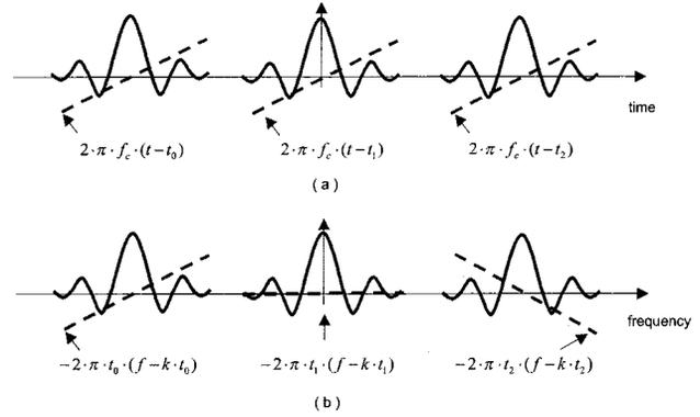
Fig. 1. Phase properties within the mainlobe of the SAR impulse response function for three targets for (a) stripmap focusing via matched filtering and (b) burst mode focusing with the SPECAN approach. The solid line gives the amplitude of the signal, and the dashed line the phase.
