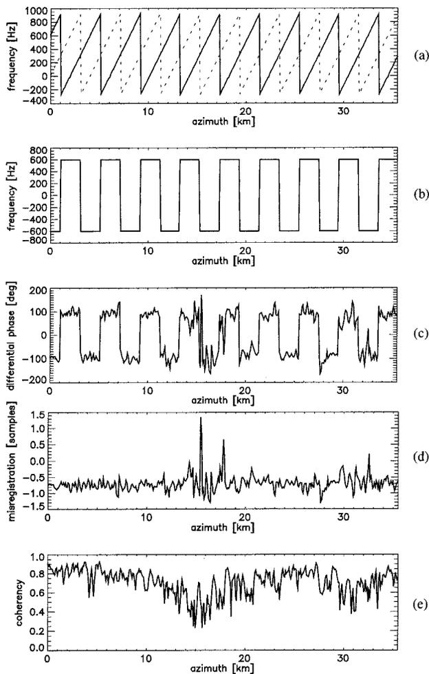
Fig. 13. (a) Azimuth frequency vector for look 1 (solid line) and look 3 (dashed line) of the simulated ScanSAR operation mode. (b) Frequency difference (look separation) as a function of azimuth position. (c) Difference phase between look 1 and 3 [horizontal cut through Fig. 12(a)]. (d) Estimated raw data burst misalignment [horizontal cut through Fig. 12(b)]. (e) Coherence information [horizontal cut through Fig. 11(c)].
