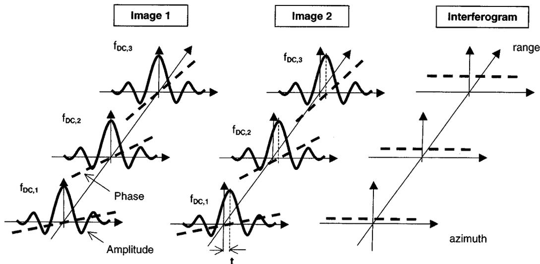
Fig. 2. Misregistered interferometric signal pair prior to interferogram generation. Range-dependent phase offsets occur due to misregistration, and the linear phase term of the IRF is imposed by the center frequency offset. When the center frequency is range dependent, the phase error due to misregistration is also range dependent.
