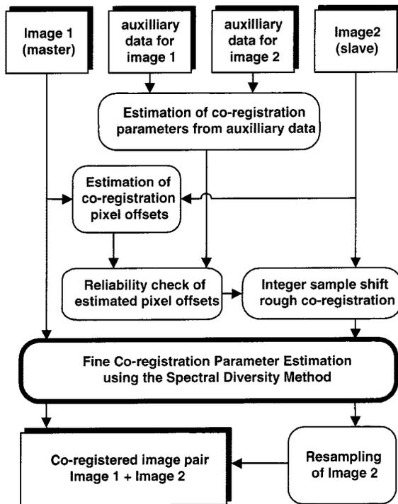
Fig. 7. Strategy for coregistration of repeat-pass interferometric data.
