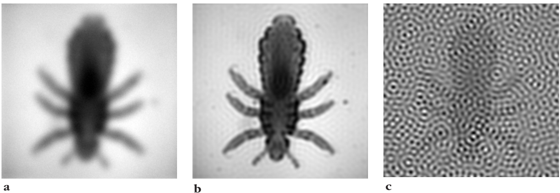
Figure 58. Effect of noise on deconvolution: (a) severely blurred image of the bug in Figure 54 with added random noise; (b) deconvolution that can be achieved in the absence of noise; (c) deconvolution with noise present.
