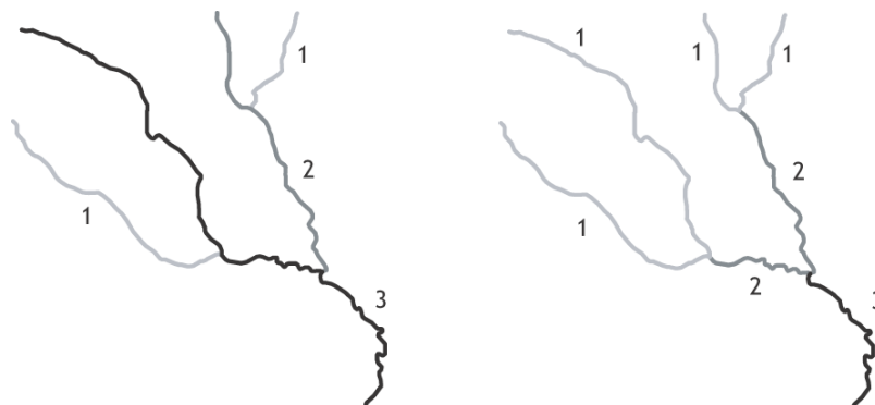
Figure 4.1: The Horton (left) and Strahler ordering (right) of hydrologic networks. Data: VECTOR200 © swisstopo (BA034957).
