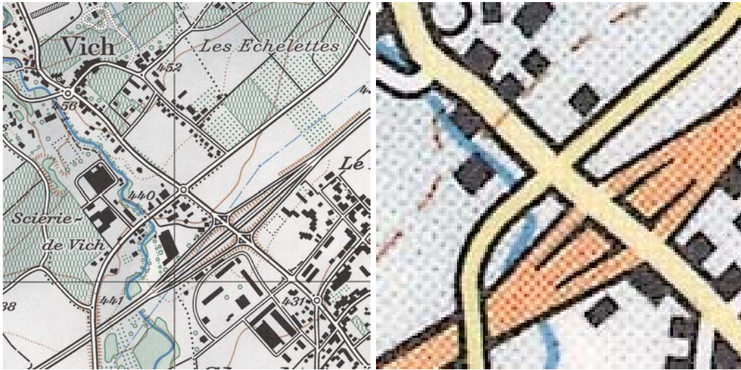
Figure 5.1: Excerpt of the Swiss national maps of 1:25'000 (left) and 1:200'000 (right, magnified to 1:25'000) illustrating the different representations of the road network of the same area (not to scale). Data: © swisstopo (BA034957).
