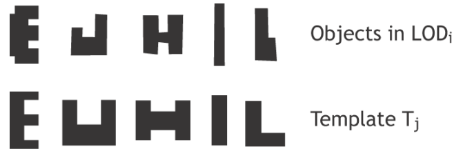
Figure 4.3: Describing outlines of building objects by using alphabetic characters or templates defined beforehand.
